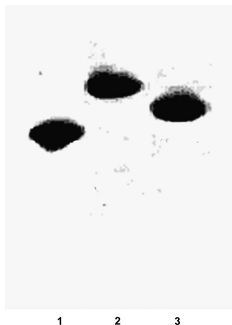
Figure 5 Native PAGE analysis of CHD-lysozymes. Native PAGE was performed on 15% gel and stained with Coomassie Brilliant Blue. Lane 1, egg white lysozyme; lane 2, CHD-lysozyme with three modified Arg residues; lane 3, CHD-lysozyme with two modified Arg residues
